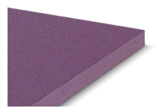
A mixed-cell polyurethane foam designed specifically for vibration and structure-borne sound isolation. Offers outstanding internal damping and low frequency isolation at minimal deflection and comes in a standard thickness of 25mm (1"). Can be installed in multiple layers to achieve a greater total thickness.
